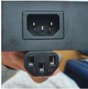
A picture of an IEC C14 power input port on a computer power supply.
